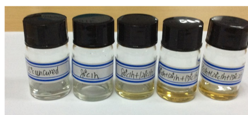
(a) Cured with MHHPAN accelerated by N -benzyl dimethylamine
